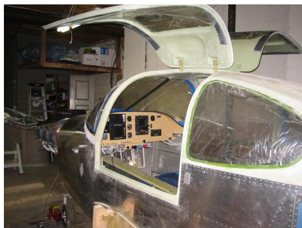
Now, at about 800 hours (spread over about a year and a half of wall clock time), the avionics and panel are done, electrical systems in, engine and prop are on, and the gull wing doors with their silly rabbit ear appearance, are shaping up with lots of sanding and filling.
