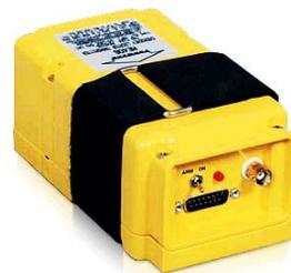
Transmitter (ELT). It broadcasts a signal on 121.5 and 243.0 MHz when activated either manually or automatically by a crash activated device. All aircraft are required to have one. The only
