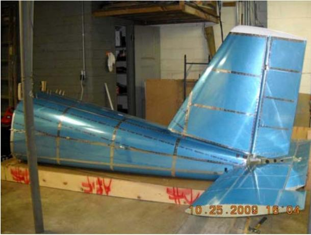
of 65 shop hours, and more than a third of that was spent prepping and priming the internal pieces with a Boeing-style two-part epoxy primer, which is entirely my preference (since this bird will live very close to salt water in a marine climate). Many builders can and do dispense entirely with priming, and get long-lived airframes just by riveting the parts together as they come out of the box.
