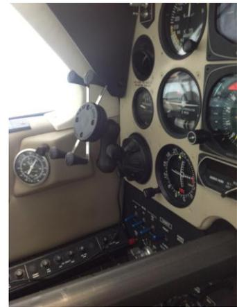
This setup needs external power. When Xavion is running, the iPhone is always on so the battery will not last long. I've added another USB supply to take care of that.
